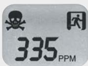
The LCD displays the level of CO in ppm, faults, status and recommended actions. The level of CO will start flashing on the LCD display as soon as the Alarm detects 10ppm. (CO levels are displayed up to 995ppm in 5ppm intervals)
